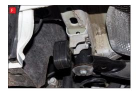
A) Both of the rear mounting points need rotating 180° when fitting the Scorpion exhaust.
